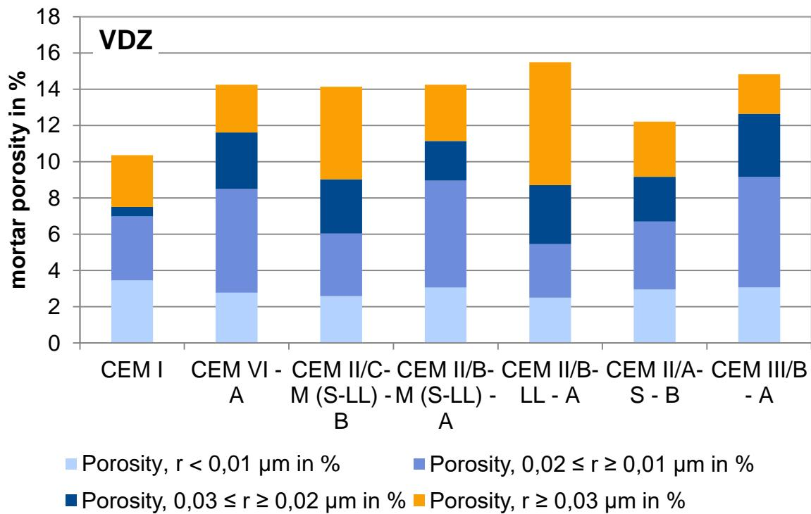
**Figure 5** Porosity of standard mortars (VDZ)
