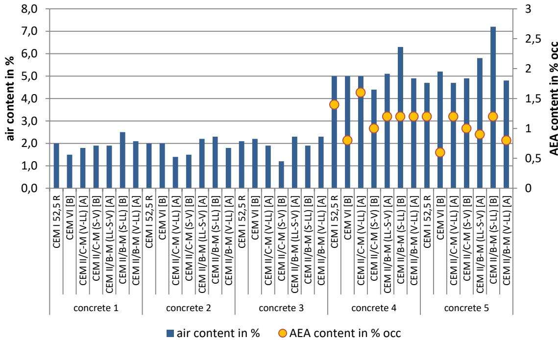
**Figure 14** Fresh concrete air contents of concretes C1 – C5 (SMG)
