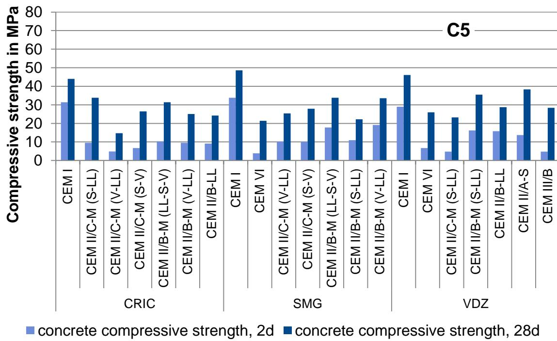
**Figure 21** Compressive strengths of concretes C5
