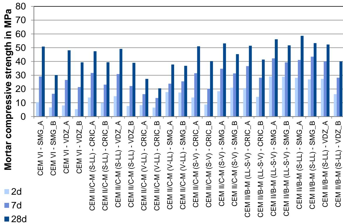
**Figure 2** Mortar compressive strength of laboratory cements (1)
