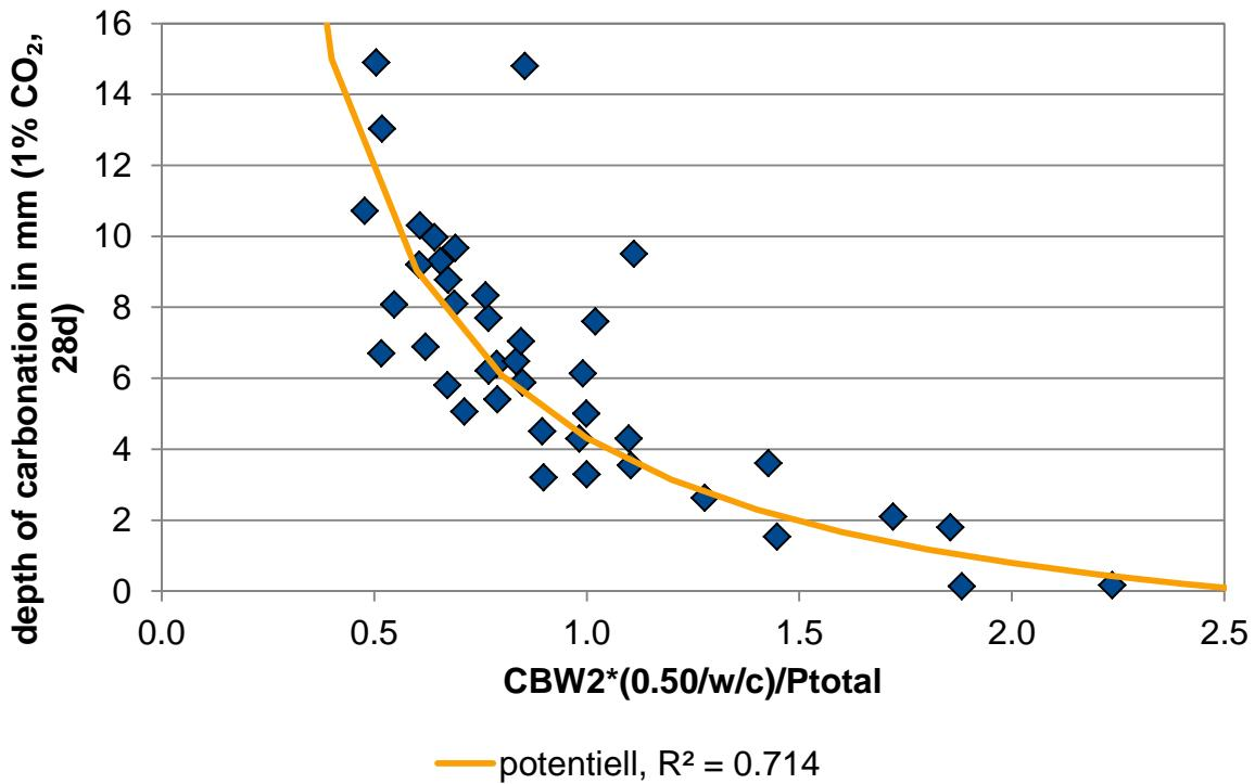
**Figure 40** Characteristic value vs. depth of carbonation acc. to EN 13295
