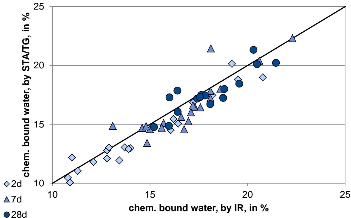
**Figure 4** Comparison of chemical bound water determined by STA and IR
