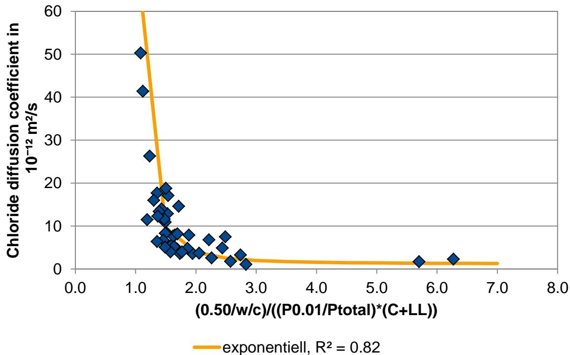
**Figure 45** Characteristic value vs. Chloride diffusion coefficient
