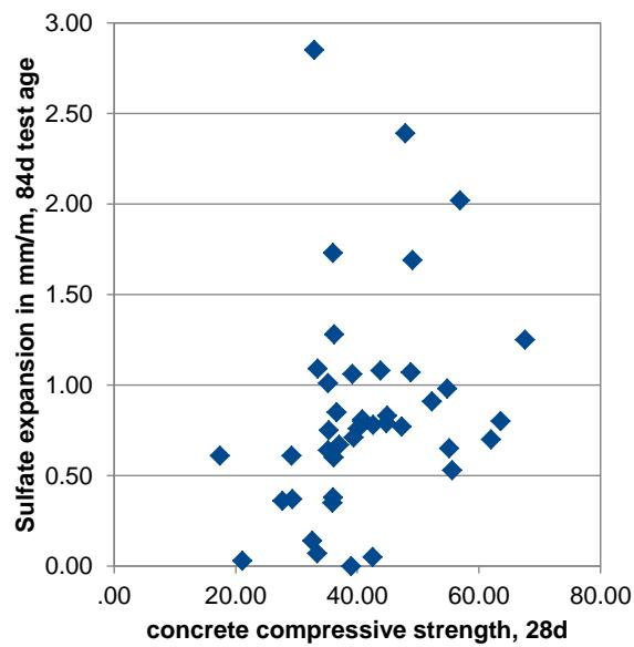
**Figure 53** Concrete compressive strength (28d) vs. expansion at the end of sulphate testing
