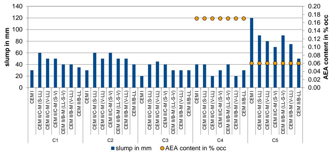
**Figure 15** Slump of concretes C1 – C5 (CRIC)
