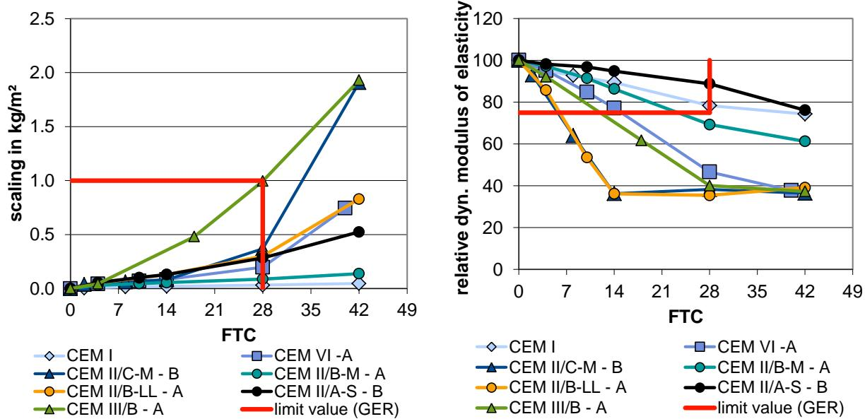
Figure 28 Scaling and the relative modulus of elasticity (VDZ)
