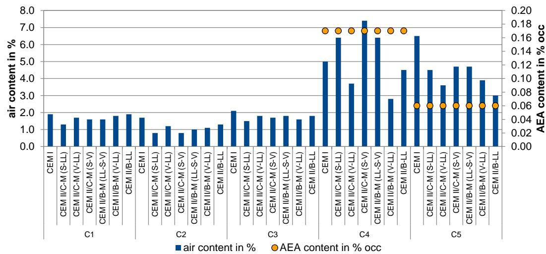
**Figure 16** Fresh concrete air contents of concretes C1 – C5 (CRIC)
