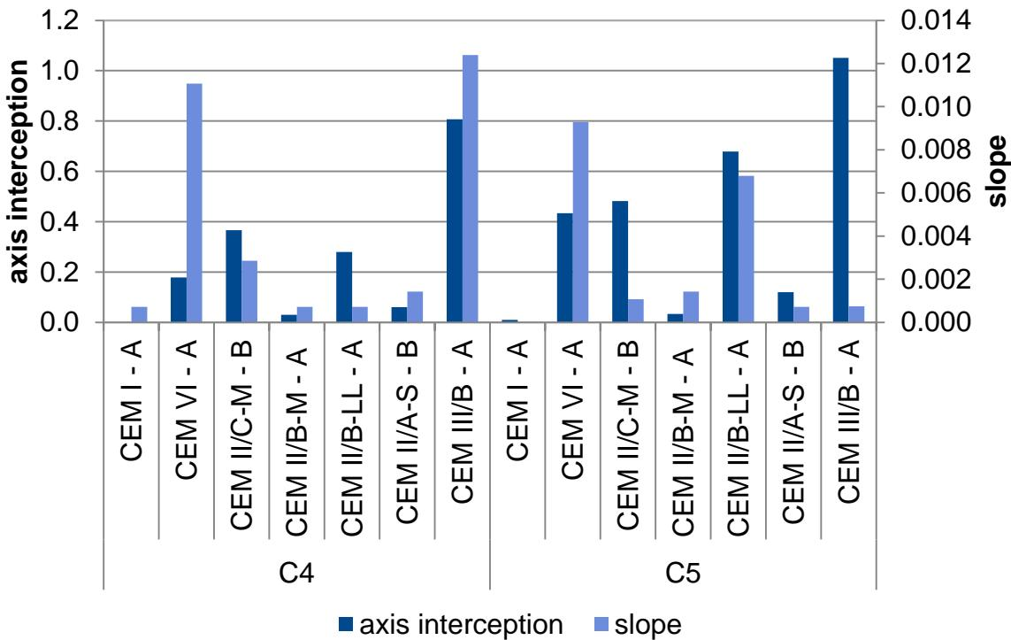
**Figure 35** Surface scaling and the speed of scaling (VDZ)
