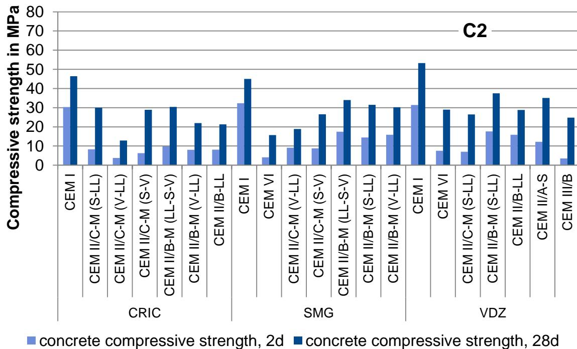
**Figure 18** Compressive strengths of concretes C2
