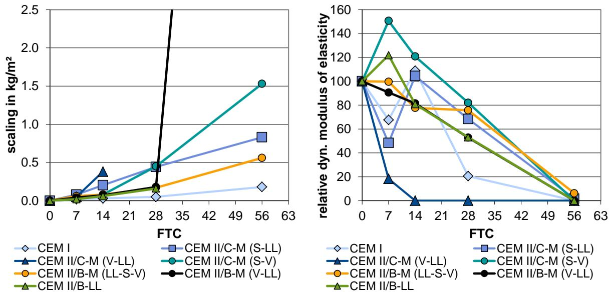
**Figure 30** Scaling and the relative modulus of elasticity (CRIC)
