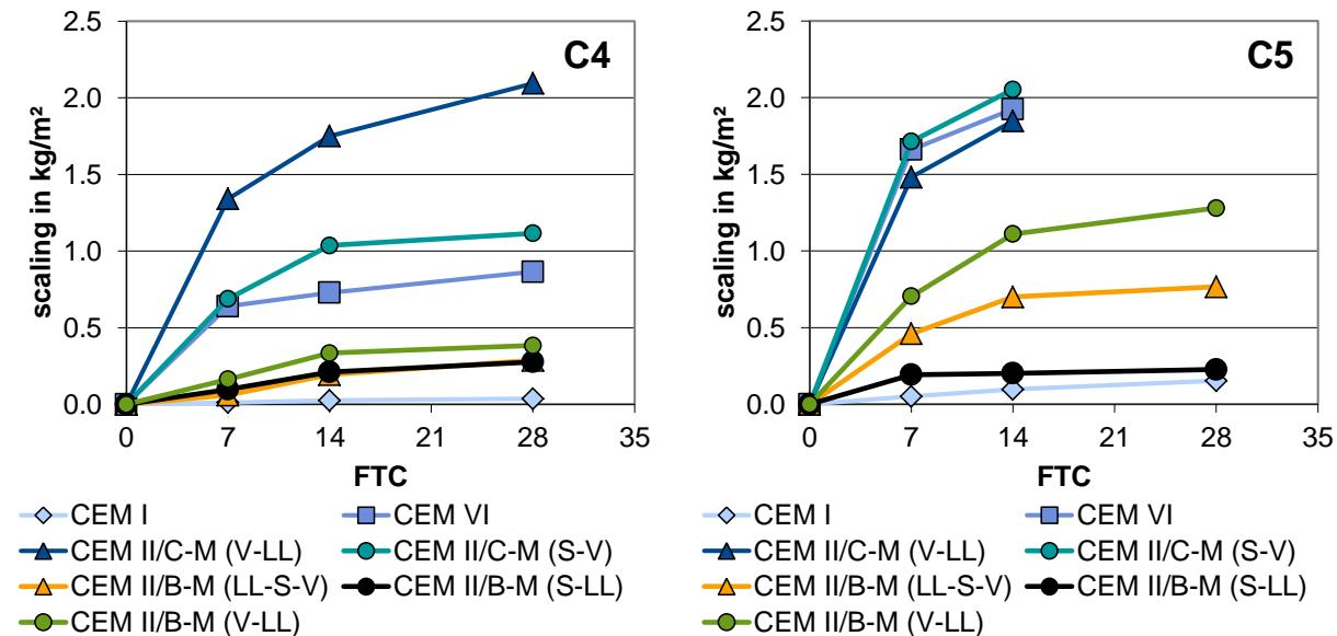
**Figure 32** Scaling with de-icing salts (SMG)
