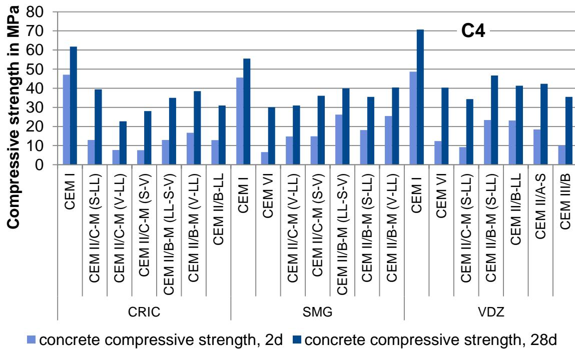
**Figure 20** Compressive strengths of concretes C4
