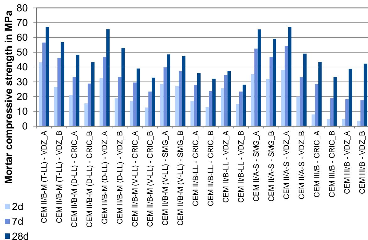
**Figure 3** Mortar compressive strength of laboratory cements (2)
