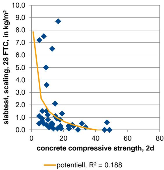
**Figure 49** Concrete compressive strength (2d) vs. scaling in the slab test
