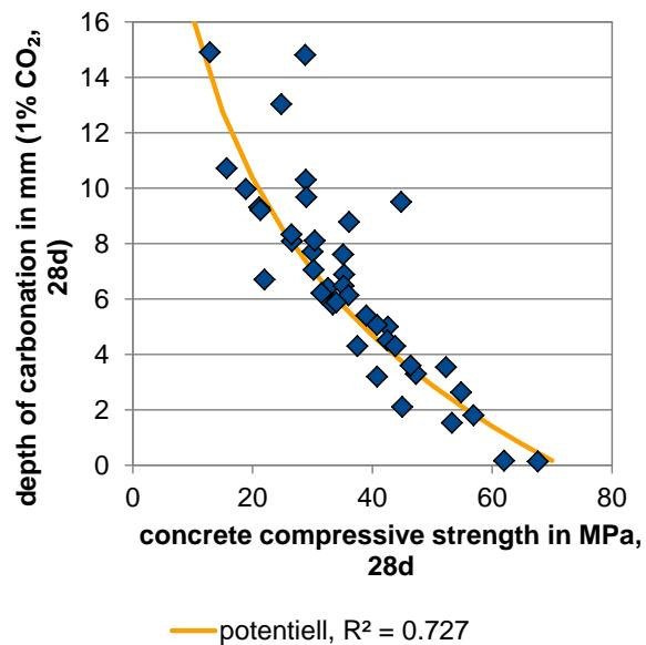
**Figure 39** Concrete compressive strength (28d) vs. depth of carbonation acc. to EN 13295
