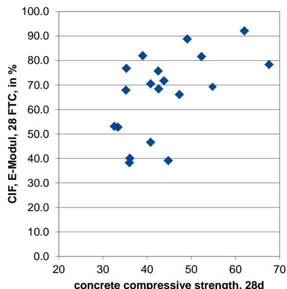
**Figure 47** Concrete compressive strength (28d) vs. relative dynamic modulus of elasticity after 28 FTC
