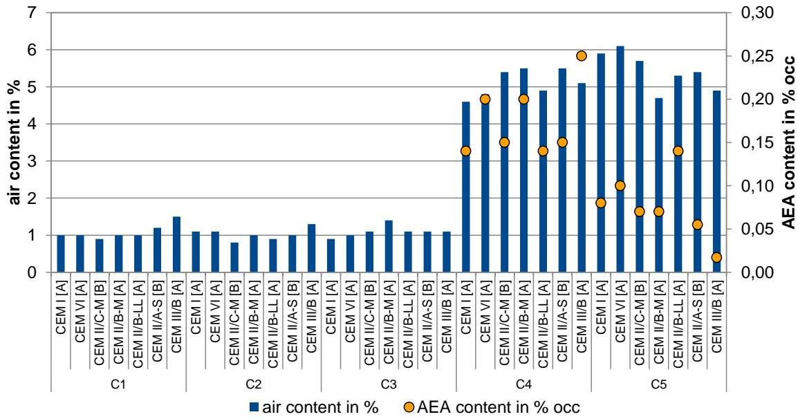
**Figure 12** Fresh concrete air contents of concretes C1 – C5 (VDZ)
