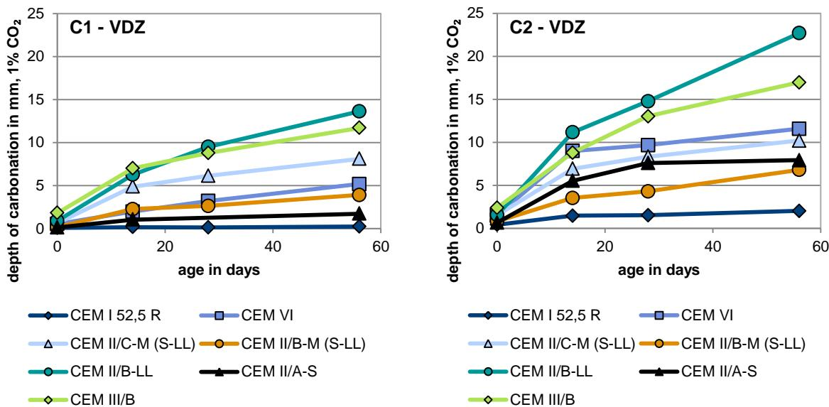
**Figure 22** Carbonation depth of concretes C1 and C2 (VDZ)
