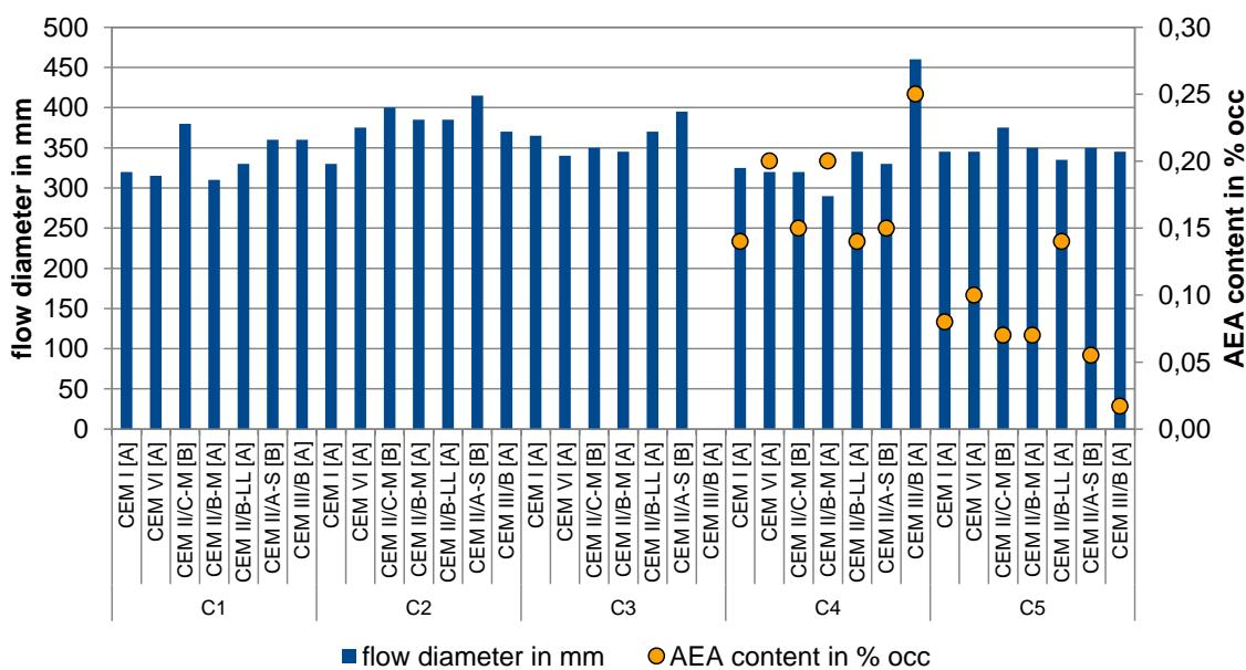
**Figure 11** Flow diameters of concretes C1 – C5 (VDZ)
