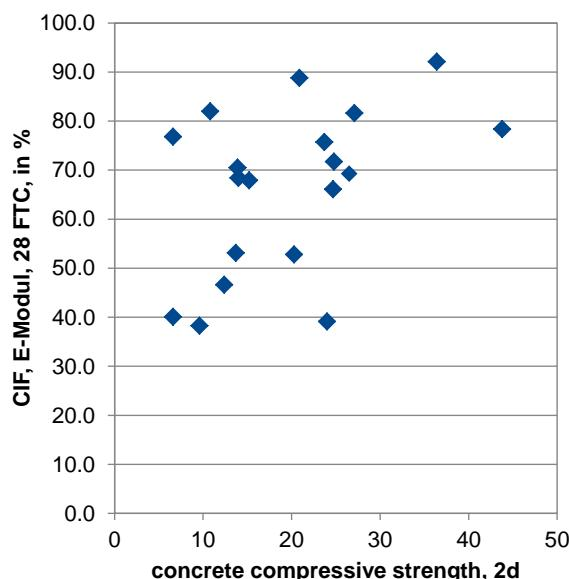
**Figure 46** Concrete compressive strength (2d) vs. relative dynamic modulus of elasticity after 28 FTC
