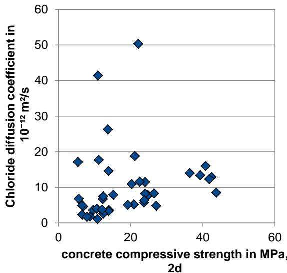
**Figure 41** Concrete compressive strength (2d) vs. Chloride diffusion coefficient
