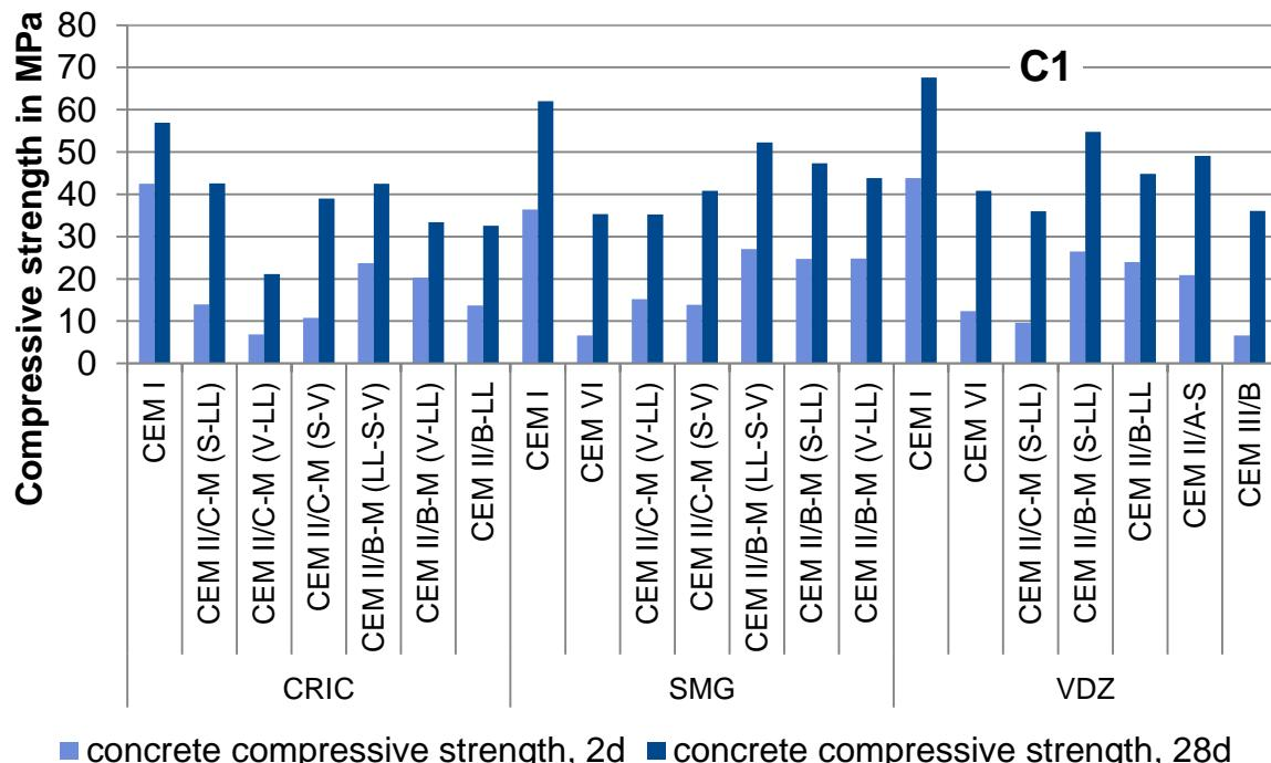
**Figure 17** Compressive strengths of concretes C1
