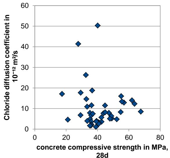
**Figure 42** Concrete compressive strength (28d) vs. Chloride diffusion coefficient
