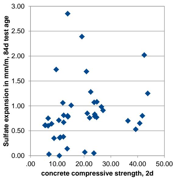
**Figure 52** Concrete compressive strength (2d) vs. expansion at the end of sulphate testing
