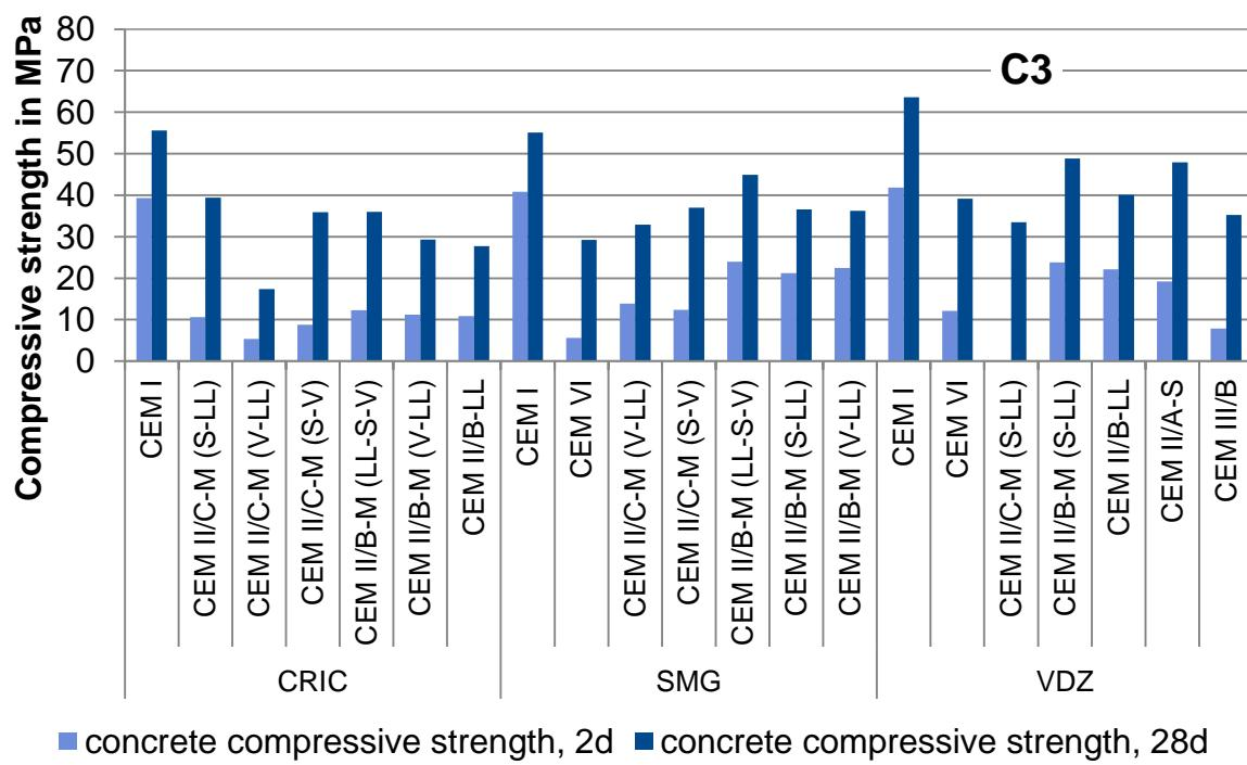
**Figure 19** Compressive strengths of concretes C3
