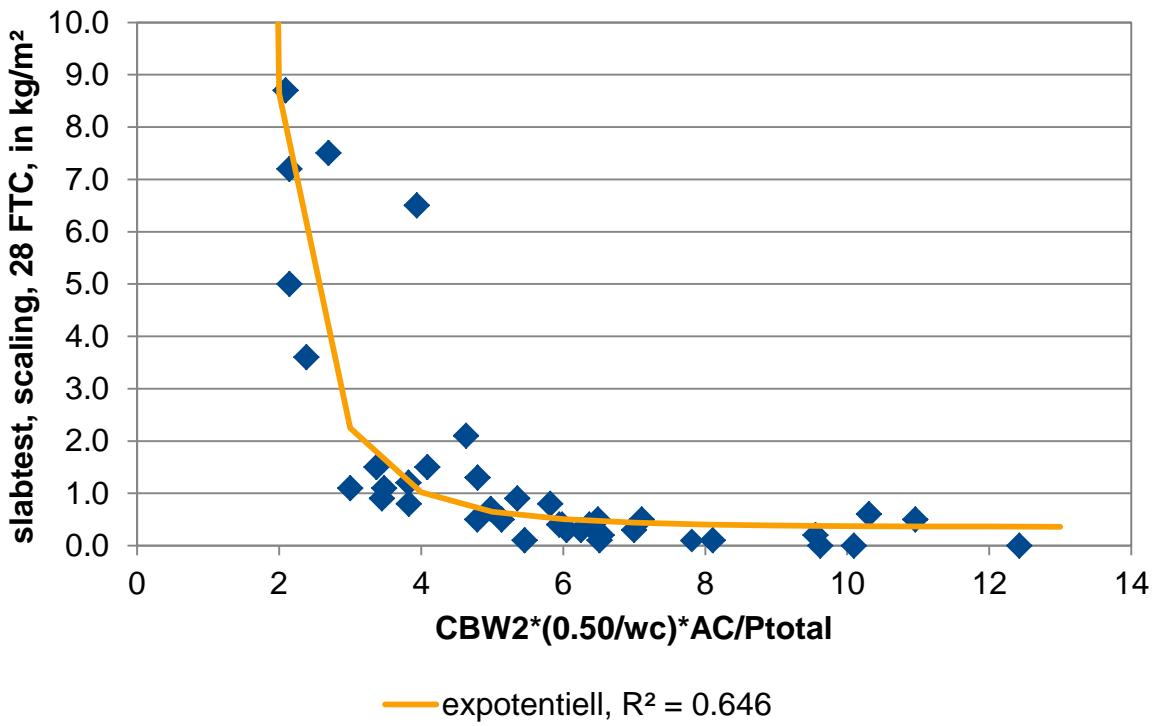
**Figure 51** Characteristic value vs. scaling in the slab test
