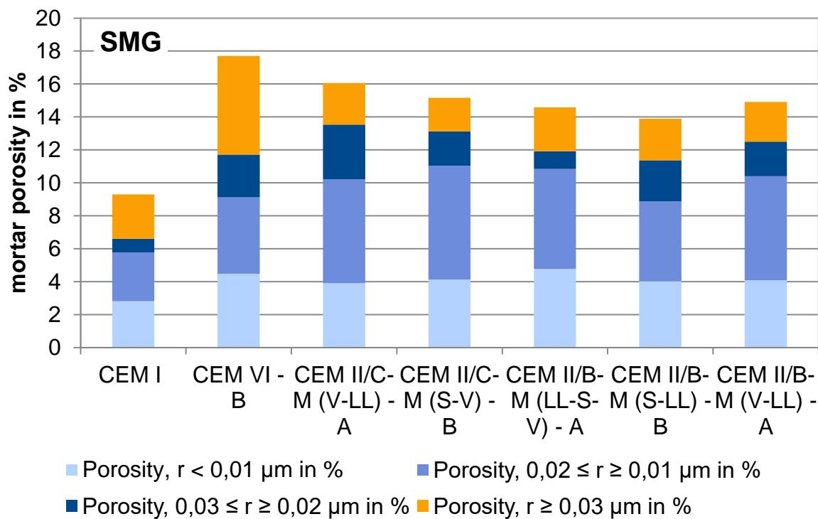
**Figure 6** Porosity of standard mortars (SMG)
