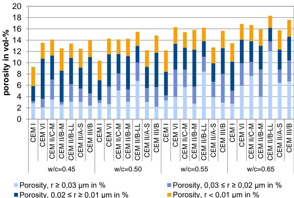
**Figure 8** Porosity of mortars with different w/c ratios (VDZ)
