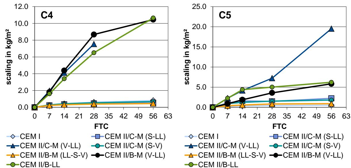
**Figure 33** Scaling with de-icing salts (CRIC)
