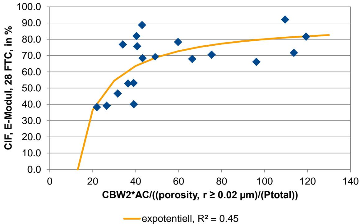
**Figure 48** Characteristic value vs. relative dynamic modulus of elasticity after 28 FTC
