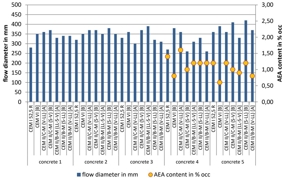
**Figure 13** Flow diameters of concretes C1 – C5 (SMG)
