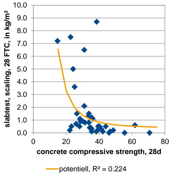
**Figure 50** Concrete compressive strength (28d) vs. scaling in the slab test
