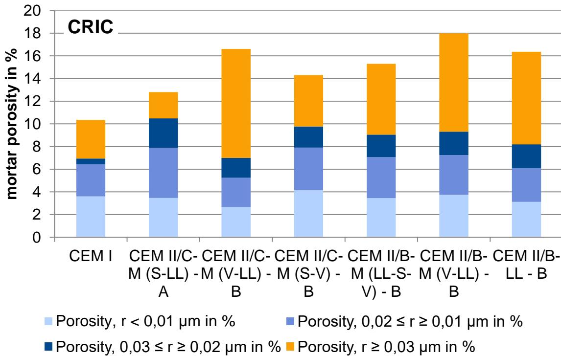
**Figure 7** Porosity of standard mortars (CRIC)
