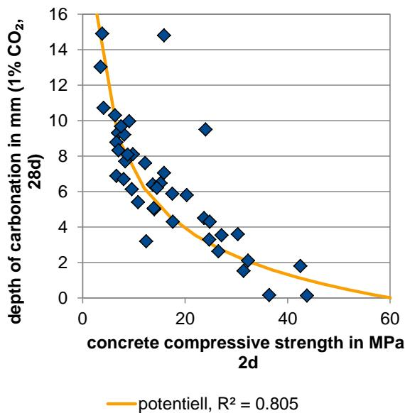
**Figure 38** Concrete compressive strength (2d) vs. depth of carbonation acc. to EN 13295
