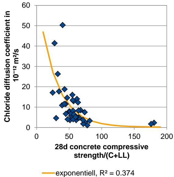
**Figure 44** Concrete compressive strength (28d)/( $\text{C}+\text{LL}$ ) vs. Chloride diffusion coefficient
