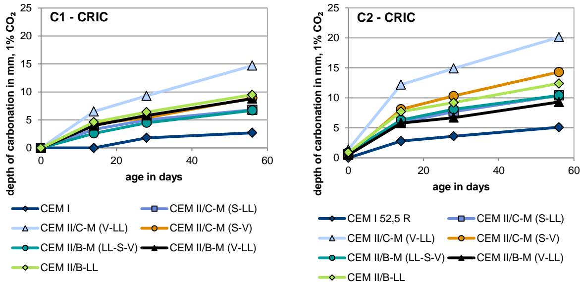
**Figure 24** Carbonation depth of concretes C1 and C2 (CRIC)
