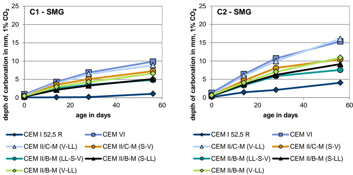
**Figure 23** Carbonation depth of concretes C1 and C2 (SMG)
