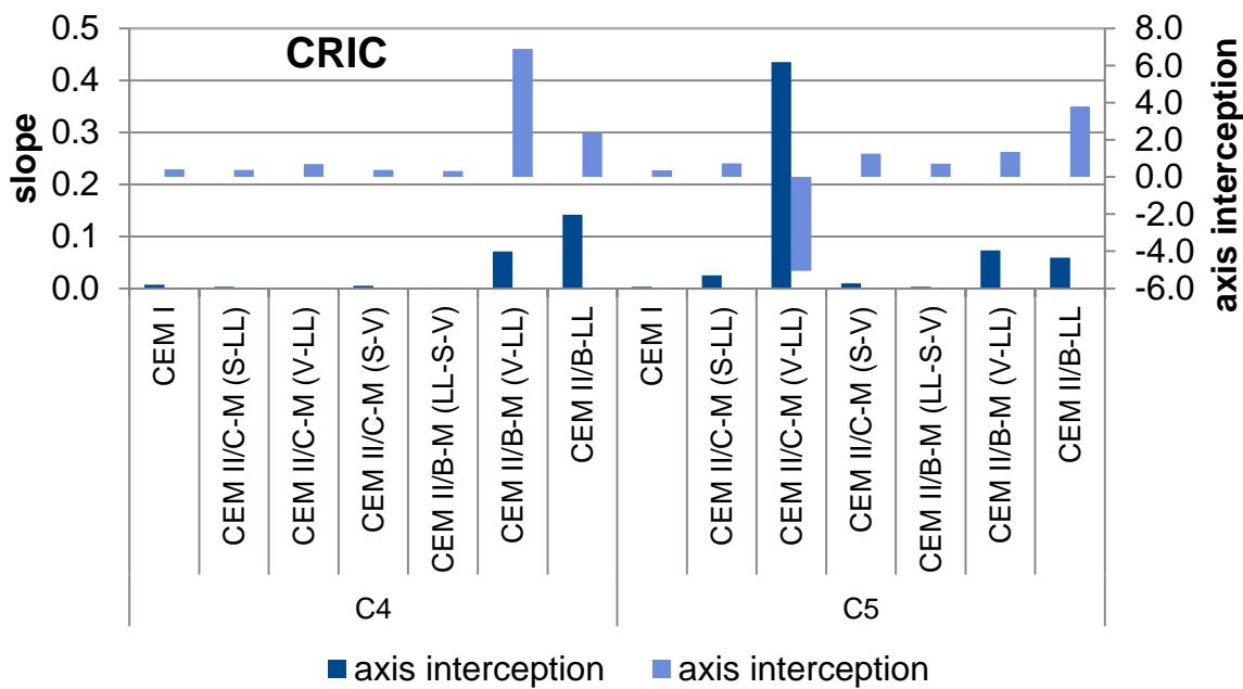
**Figure 37** Surface scaling and the speed of scaling (CRIC)
