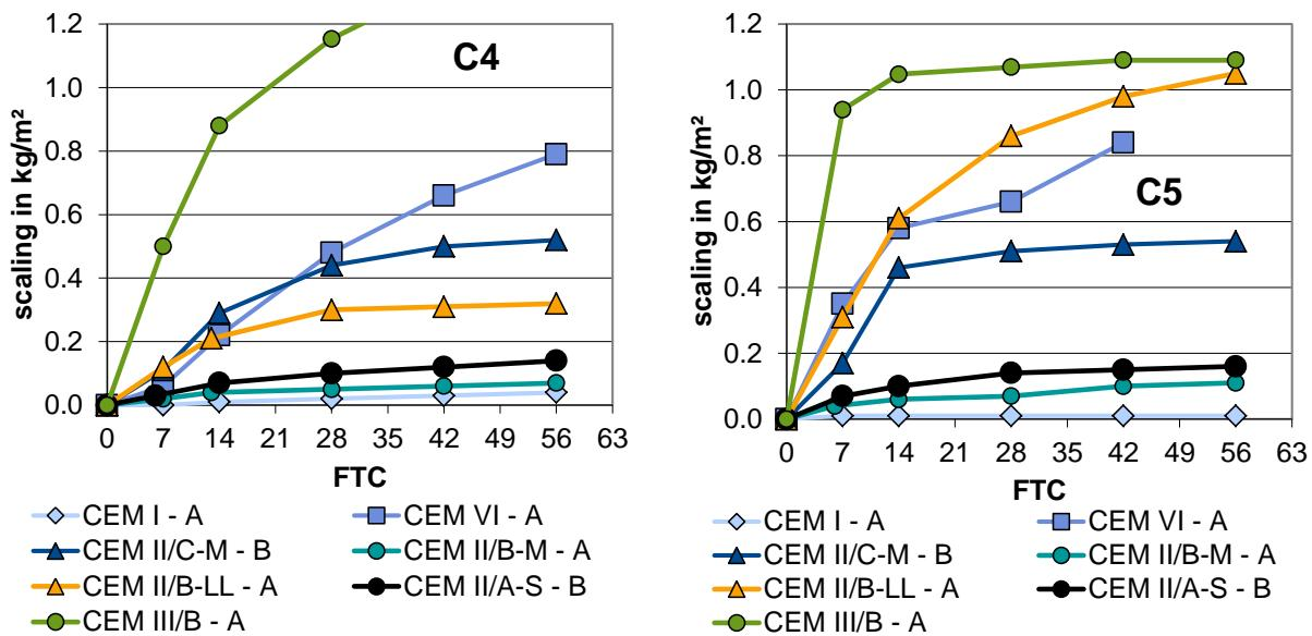
**Figure 31** Scaling with de-icing salts (VDZ)
