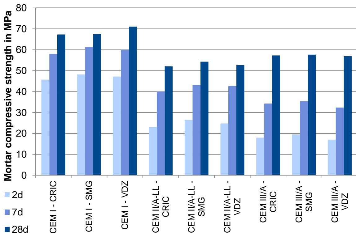
**Figure 1** Mortar compressive strength of reference cements
