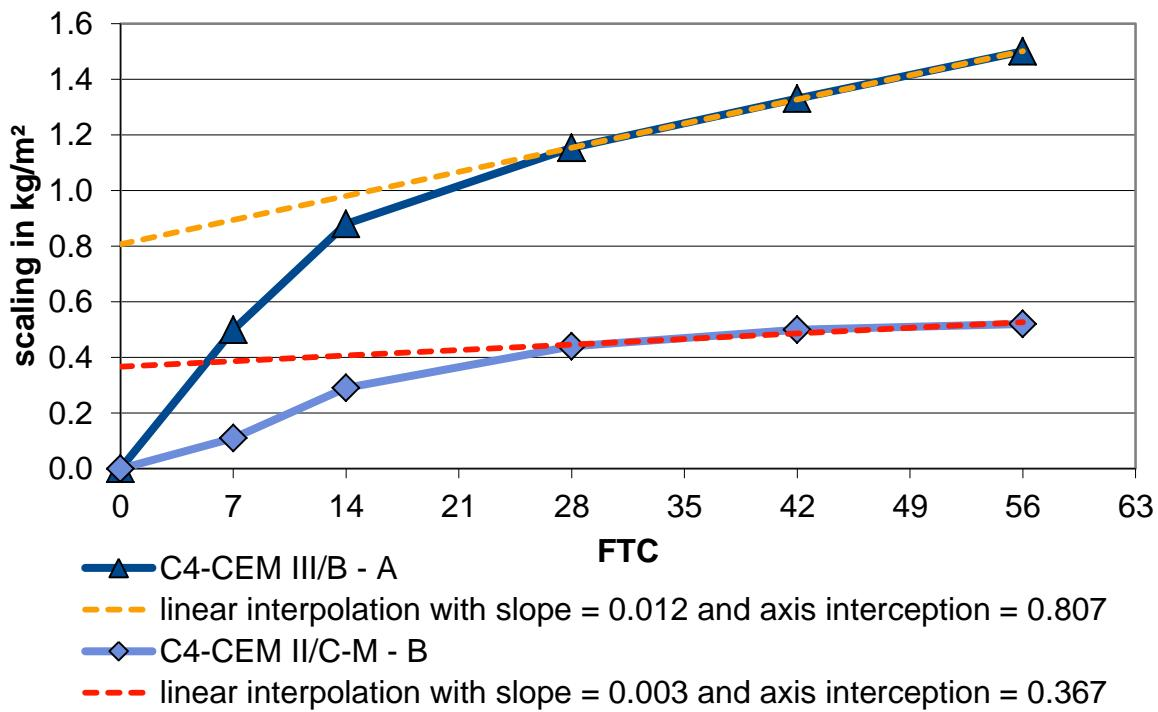
**Figure 34** Surface scaling and the speed of scaling (principle)
