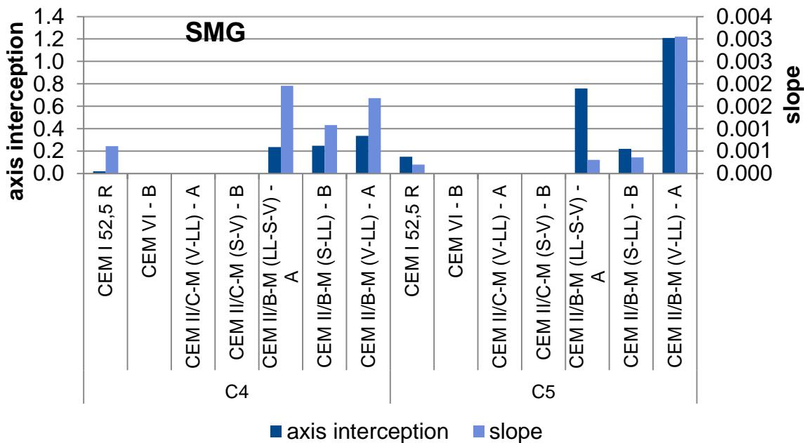
**Figure 36** Surface scaling and the speed of scaling (SMG)
