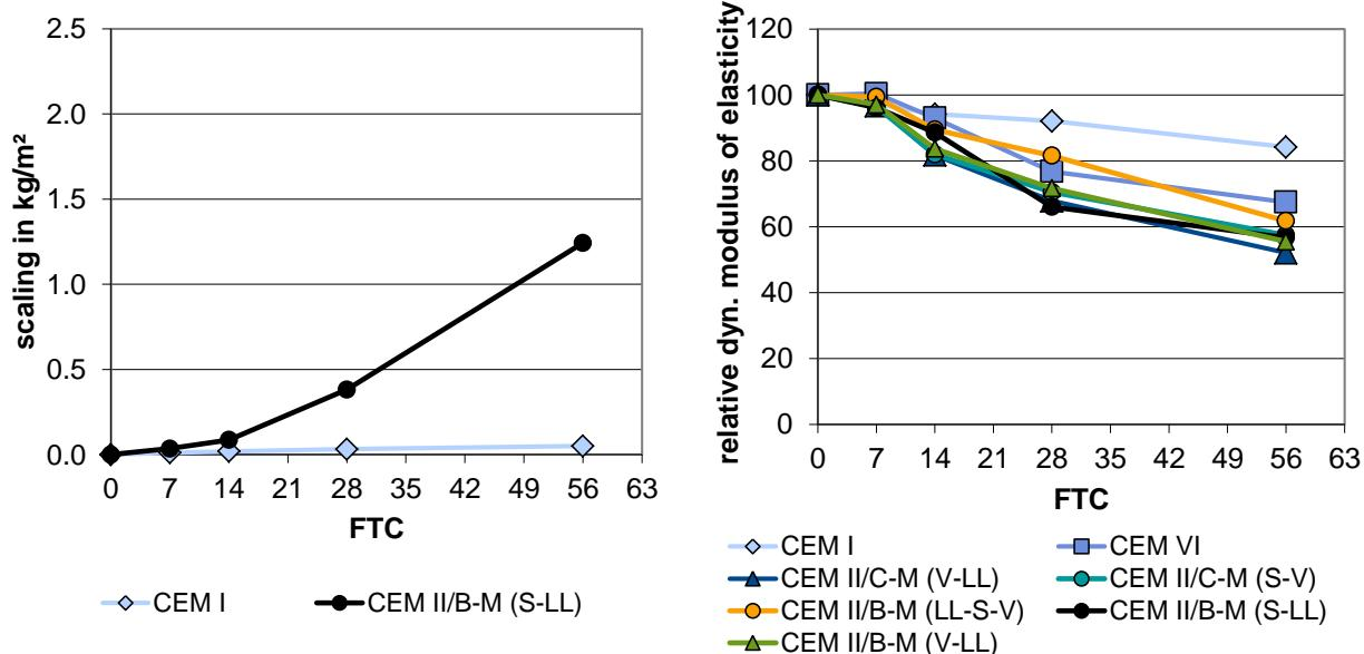
Figure 29 Scaling and the relative modulus of elasticity (SMG), RDM calculated from XF3 testing according to ONR23303; correlated with CIF tests from the CIF results of CEM I and CEMII/B-M(S-LL)
