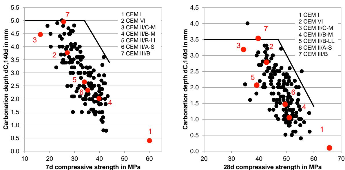
**Figure 25** Carbonation depth of fine concretes (VDZ)
