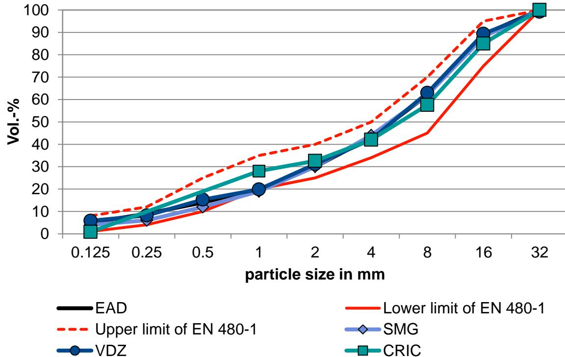
**Figure 10** Grading curves of aggregates used in the project
