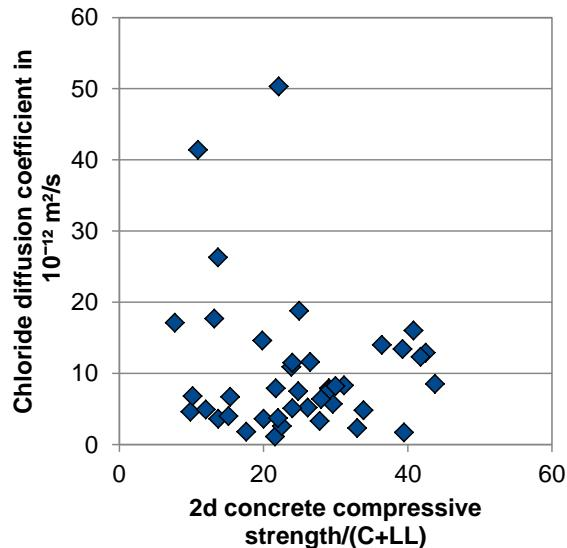
**Figure 43** Concrete compressive strength (2d) /( $\text{C}+\text{LL}$ ) vs. Chloride diffusion coefficient
