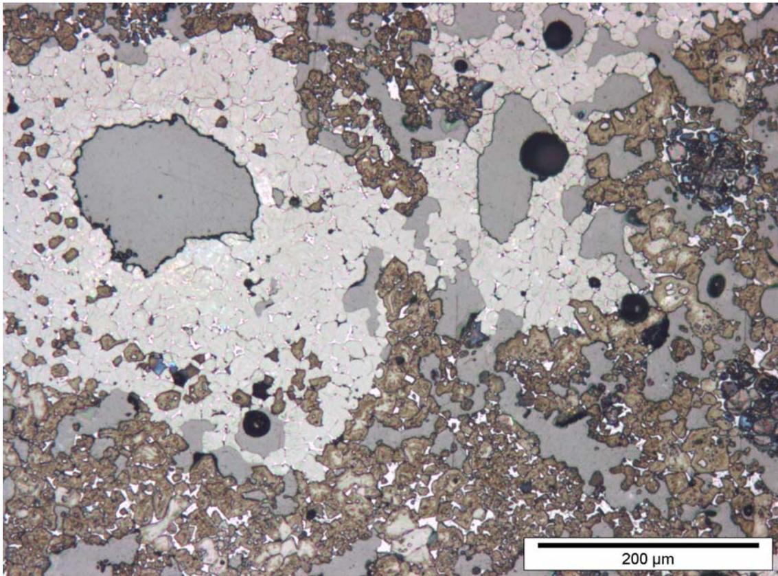
Figure 1: Belite clusters with central pores
