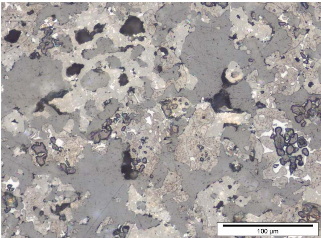
Figure 4: Porous clinker resulting from intermediate burning
