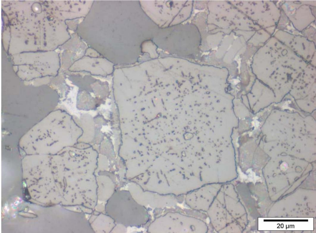
Figure 6: Alite burned in reducing atmosphere, showing partly decomposition to belite and free lime along crystallographic preferred orientations
