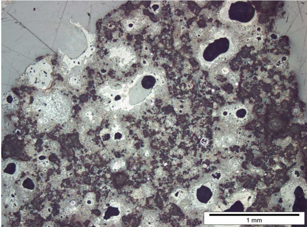
Figure 3: Belit clusters (light grey) and free lime (dark grey) in a poorly burned clinker grain
