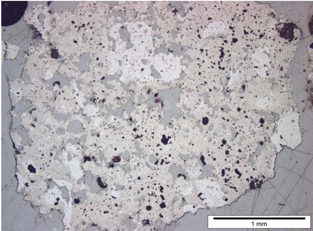
Figure 2: Well burned clinker with typical phase assemblage and few belite clusters
