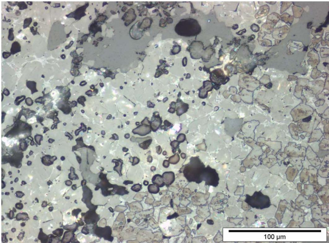
Figure 5: Belite enriched in phosphate (light grey), interspersed with fine grained free lime (dark grey)
