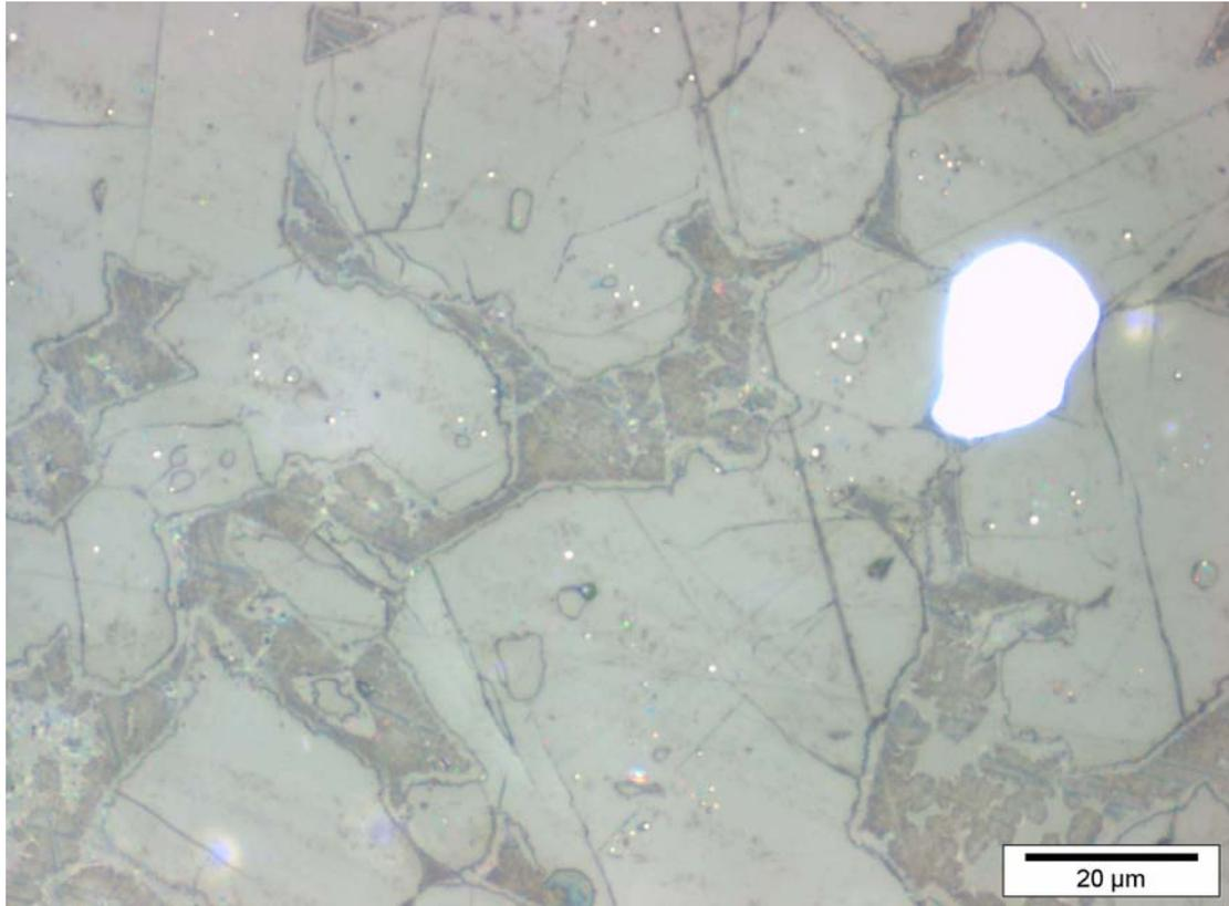
Figure 7: Metallic iron (white) forming a 20  $\mu\text{m}$  large droplet and small inclusions ( $< 1 \mu\text{m}$ ) in alite crystals
