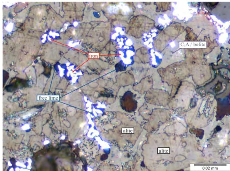
Figure 3: Reflected light micrograph of clinker; symplectites of free lime and elemental iron together with alite crystals in a ground mass free of  $C_4AF$ .
