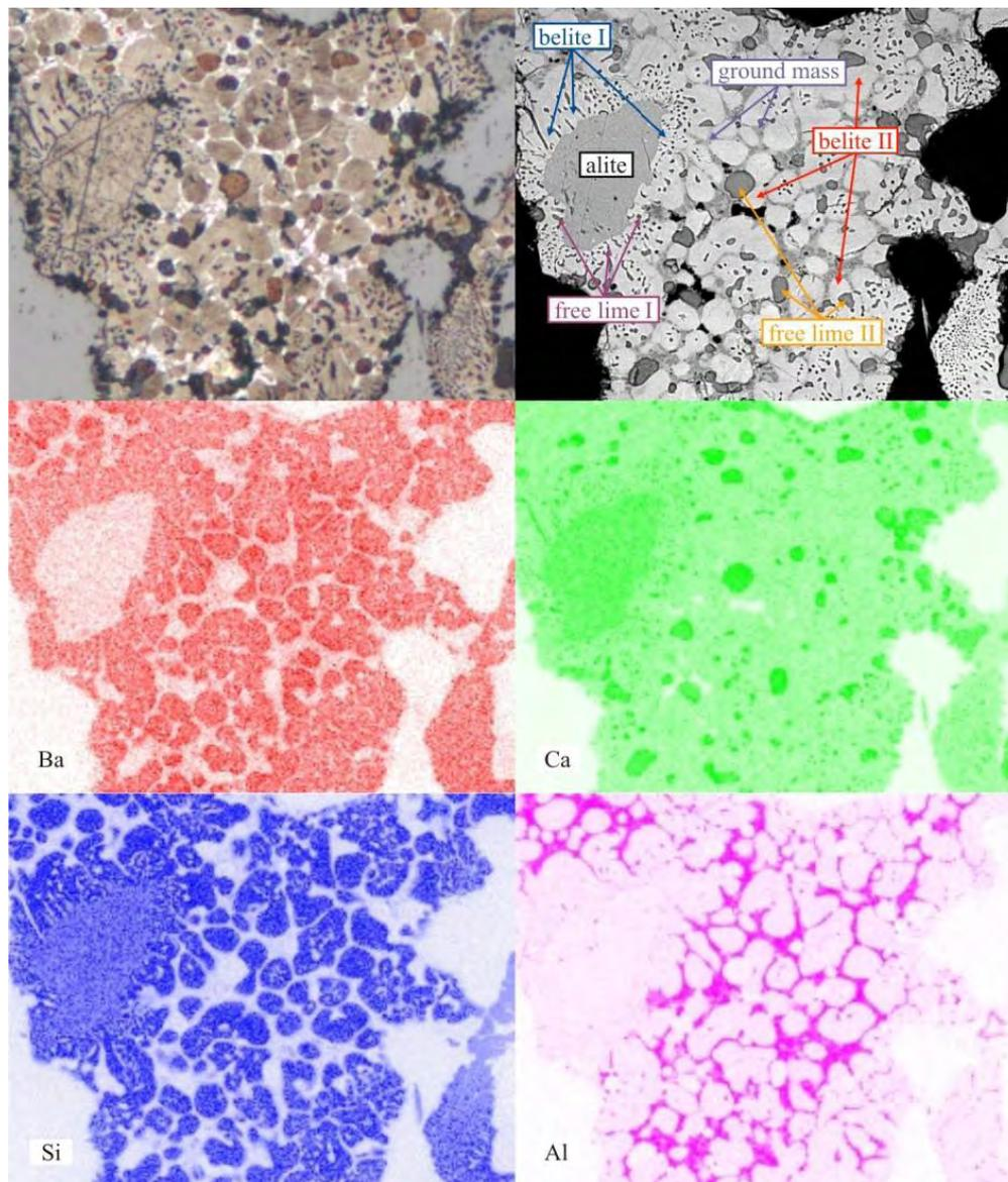
Figure 2: Reflected light (top left) and SEM micrograph (top right) of clinker; elemental maps (Ba mid left, Ca mid right, Si bottom left, Al bottom right) of alite directly surrounded symplectitic arrangement of free lime and belite, itself surrounded by a mixture of coarse free lime and belite; width of each image 235  $\mu\text{m}$ .
