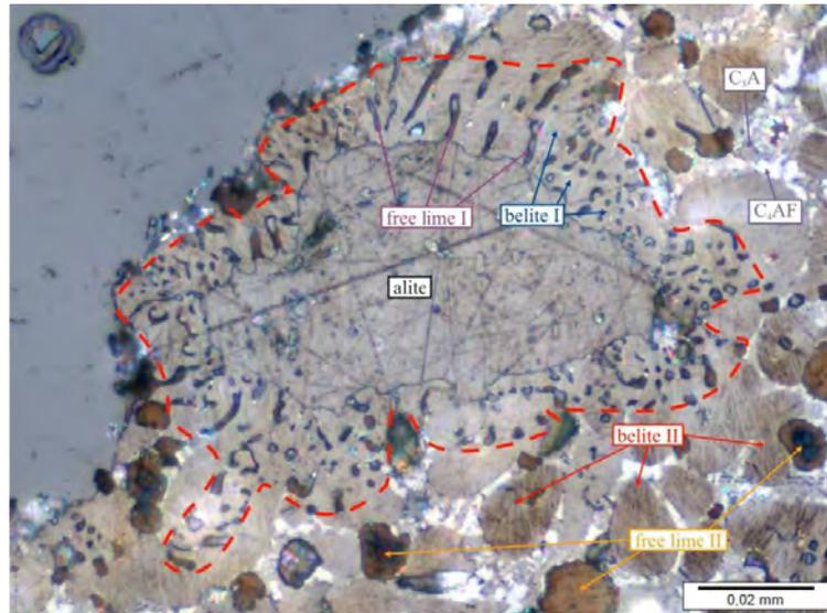
Figure 1: Reflected light micrograph of clinker; alite directly surrounded by a symplectite of free lime crystals often oriented towards alite (free lime I) and belite crystals (belite I), itself surrounded by a mixture of coarse round free lime crystals (free lime II) and belite (belite II); outer rim of symplectite marked with dashed red line.
