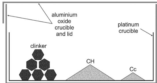
Figure 3: Setup of heating experiment for the reproduction of layers around alite crystals.
