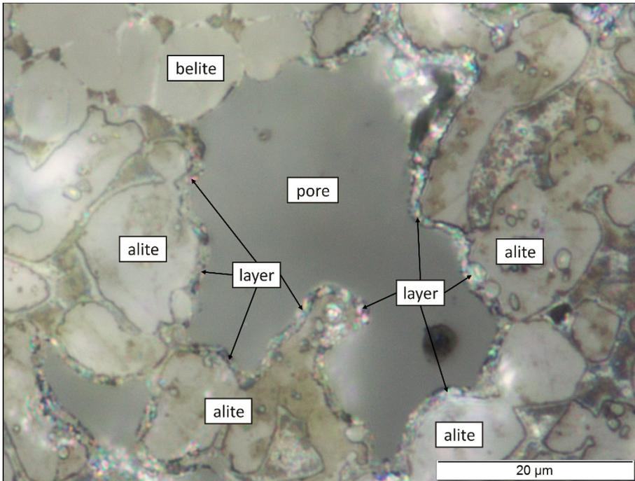
Figure 2: Layer around alite crystals in contact with pores, layer crystallinity too fine for identification.
