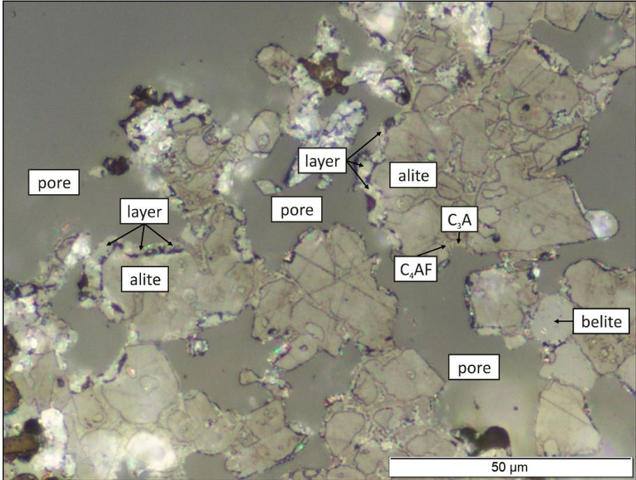
Figure 4: Layer around alite crystals in contact with pores, layer not visible on alite in contact with other solid phases or on other solid phases in contact with pores.
