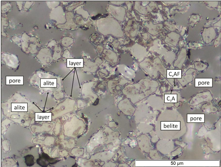
Figure 1: Layer around alite crystals in contact with pores, layer not visible on alite in contact with other solid phases or on other solid phases in contact with pores.
