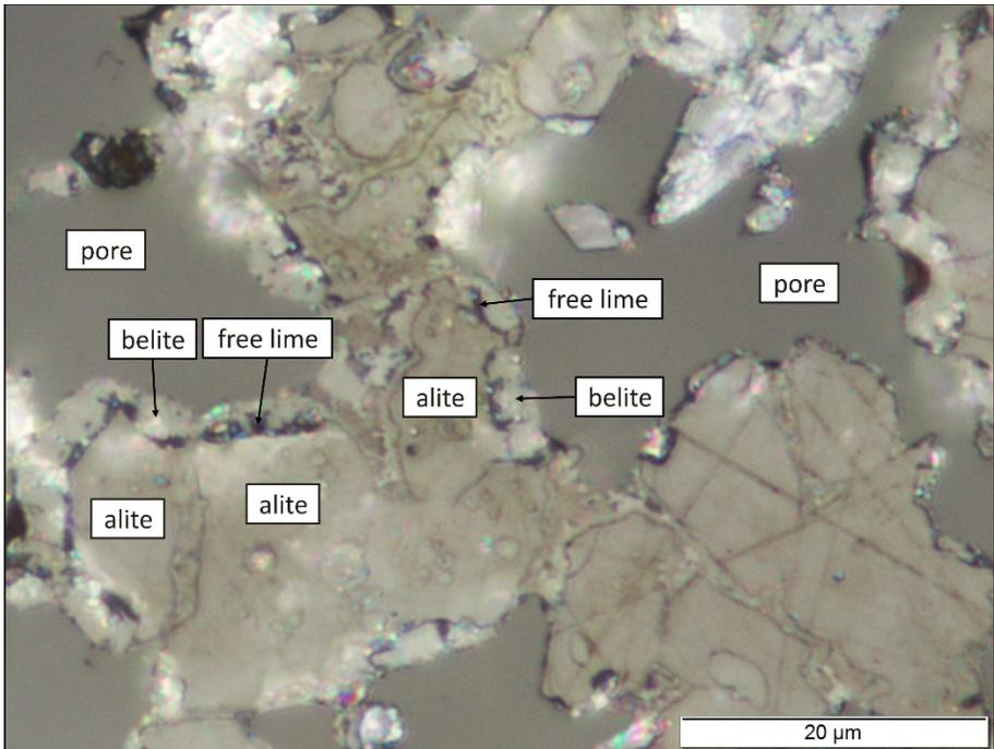
Figure 5: Layer around alite crystals in contact with pores, crystals in the layer partly identifiable as belite or free lime; detail from figure 4.
