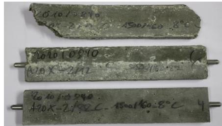
Figure 2: Mortar flat prisms based on Portland cement with 20 % fly ash, 12 month storage at 8 °C in test solution with 160 mg Mg/l after 2 days (top prism), after 14 days (central prism) and after 90 days pre-storage (bottom prism)
