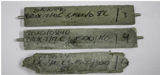
Figure 1: Mortar flat prisms based on Portland limestone cement with 20 % fly ash, 14 days pre-storage, 12 month storage at 8 °C in test solution without Mg (top prism), with 160 mg Mg (central prism) and with 300 mg Mg (bottom prism) per liter
