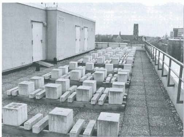
Figure 1: Prisms and cubes at the outdoor exposure site at the Research Institute in Düsseldorf
