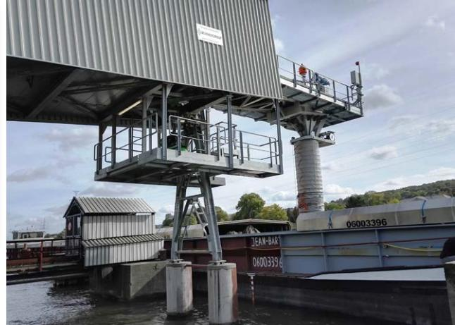
Figure 6: The Beumer Group also installed a ship loader at the end of the conveyor line. Every day, 2000 t of fly ash are loaded on to a ship
