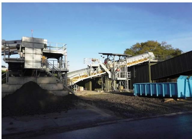
Figure 5: The material is transported from the stockpile onto the pipe conveyor
