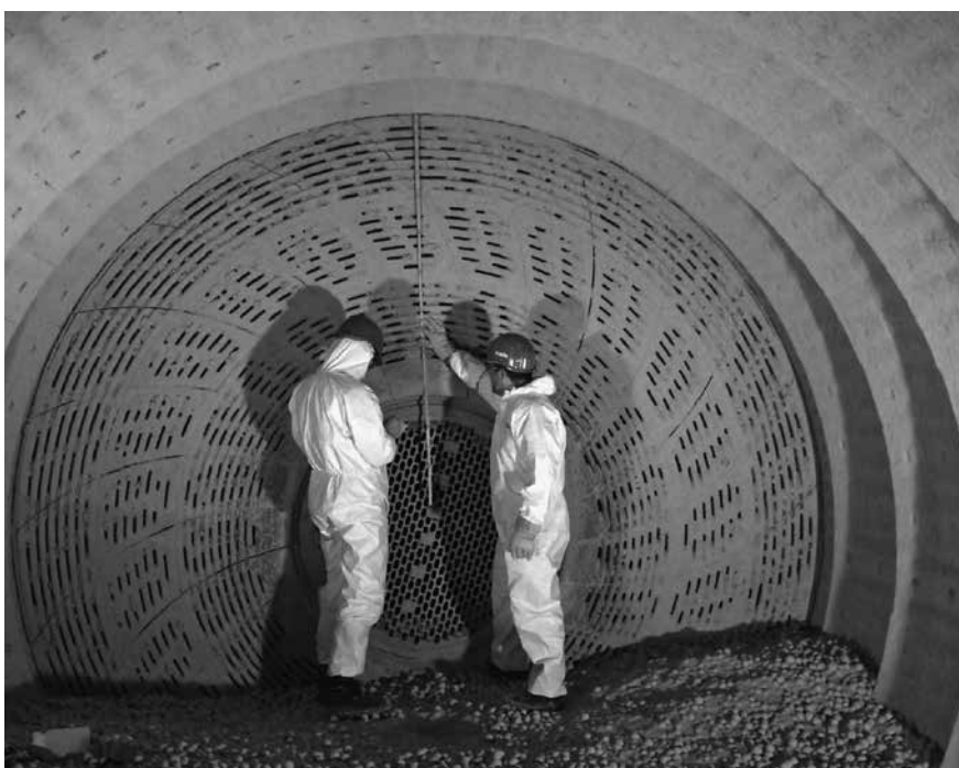
Reviewing a ball mill as part of a mill audit.
