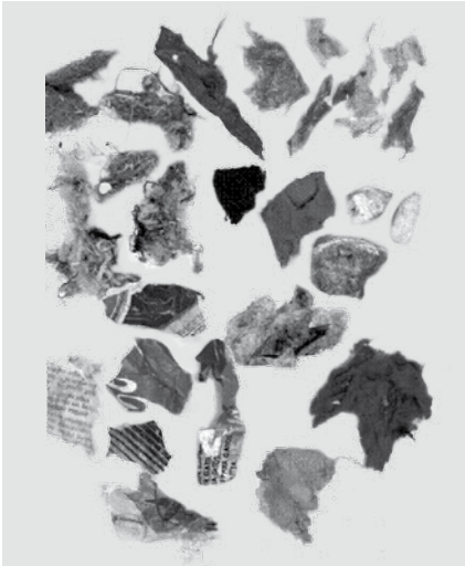
Fig. I-8: Heterogeneous composition of solid alternative fuels
