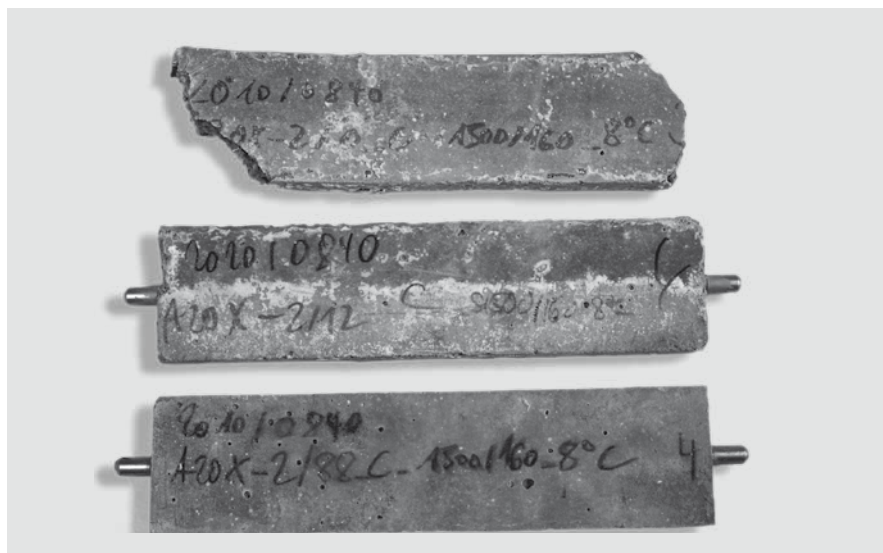
Fig. V-40: Mortar flat prisms based on Portland cement with 20% fly ash from bituminous coal, 12 months storage at 8 °C in sodium sulphate solution (S1500) with 160 mg magnesium after 2 days of preliminary storage (top prism), 14 days of preliminary storage (central prism) and 90 days of preliminary storage (bottom prism), AiF research project
