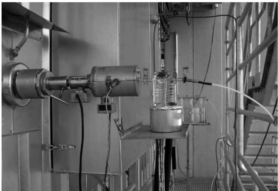
Fig. I-7: \text{SO}_3 measuring in the clean gas of a rotary cement kiln plant according to VDI directive 2462, sheet 2 (dated 2010)
