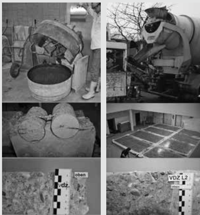
Fig. V-52: Comparison of an optimised concrete composition in the laboratory and for practical concreting in winter (CEM II/B-S 42,5 N; c = 340 \text{ kg/m}^3 ; w/c = 0.50 ; admixture: Combination of melamine and naphthalene sulphonates)
