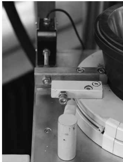
Fig. I-14: Modified measurement of power using a load cell
