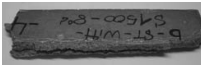
Fig. III-27: Flat mortar prism made from a binder mix consisting of 80 wt.% CEM I 32,5 R and 20 wt.% FA (w/c = 0.60, k = 1) after 18-month storage in 0.22% sodium sulphate solution at 8 °C
