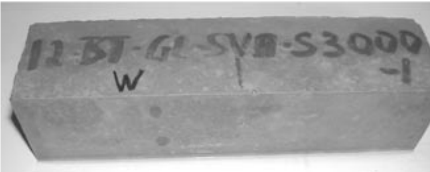
Fig. V-26: Concrete specimen ( w/c = 0.60 ) on the basis of slag cement (CEM III/B-HS) and limestone chippings after 45-month storage in 0.44% sodium sulphate solution at 8 °C
