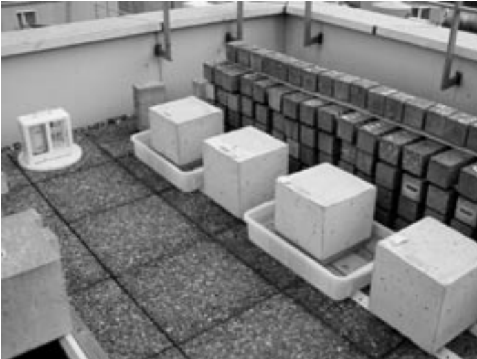
Fig. V-18: Dry and wet (footbath) out- door storage of 30 cm cubes
