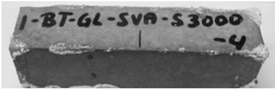
Fig. V-24: Concrete specimen (w/c = 0.60) on the basis of Portland cement (CEM I 32,5 R) and quartz gravel after 45-month storage in 0.44% sodium sulphate solution at 8 °C
