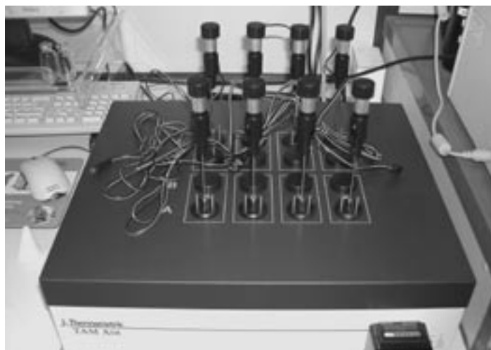
Fig. III-39: TAM Air heat flow calorimeter with 8 independent channels equipped with admix titration cells
