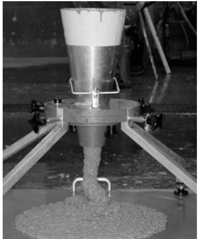
Fig. V-30: Determination of the flow time and the slump flow measure with the flow cone
