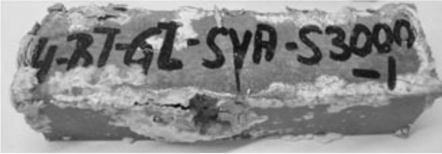
Fig. V-25: Concrete specimen ( w/c = 0.60 ) on the basis of Portland cement (CEM I 32,5 R) and limestone chippings after 45-month storage in 0.44% sodium sulphate solution at 8 °C
