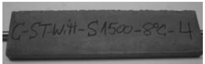
Fig. III-28: Flat mortar prism made from a binder mix consisting of 60 wt.% CEM I 32,5 R and 40 wt.% FA (w/c = 0.60, k = 1) after 18-month storage in 0.22% sodium sulphate solution at 8 °C
