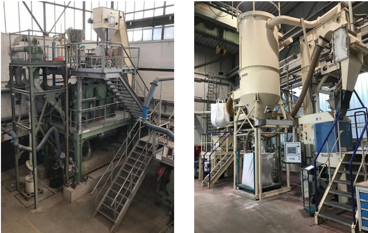
Figure 3 Left: Grinding plant with a high-pressure grinding roller for the production of coarse intermediate products from the 1 st grinding step. Right: Vertical stirred media mill, which was used for the subsequent grinding and production of the intermediate ultra-fine products from the 2 nd grinding step [Kna 2023].
