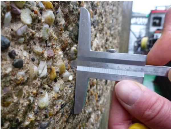
**Figure 3.** Measurement of scaling depth due to freeze-thaw attack at lock 3.
