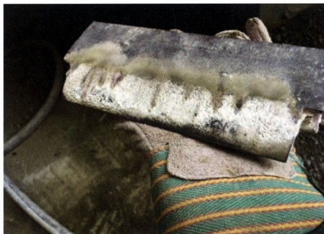
Figure 5: Dust clogging the lamellas of the cooler grate plates
