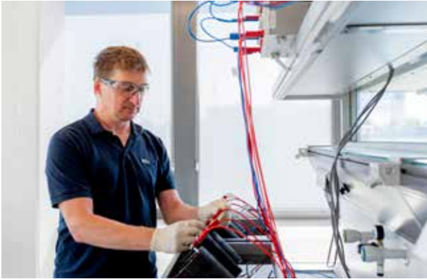
Chloride-migration testing in VDZ's laboratory
