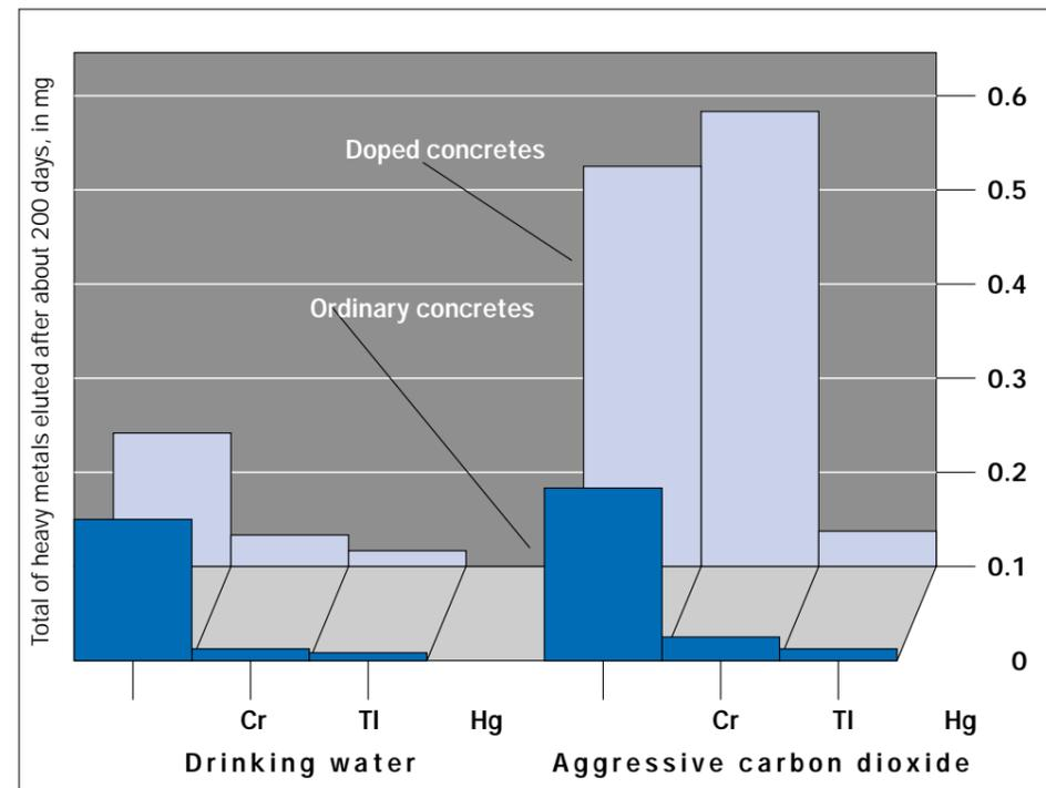
Fig. 8 Comparison of the heavy metal quantities leached from concretes after 200 days
