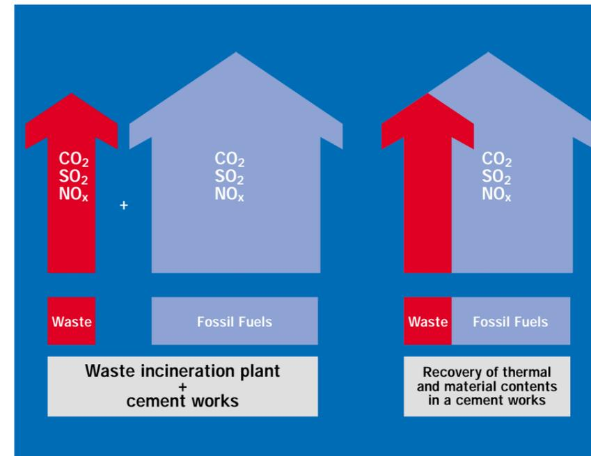
Fig. 16 Emissions and energy consumption during the clinker burning process are largely independent of the type of fuel used. If waste is therefore disposed of in plants installed for that very purpose, or reprocessed in special plants at high energy expenditure, additional emissions occur, causing a deterioration in the life cycle analysis of waste disposal.
