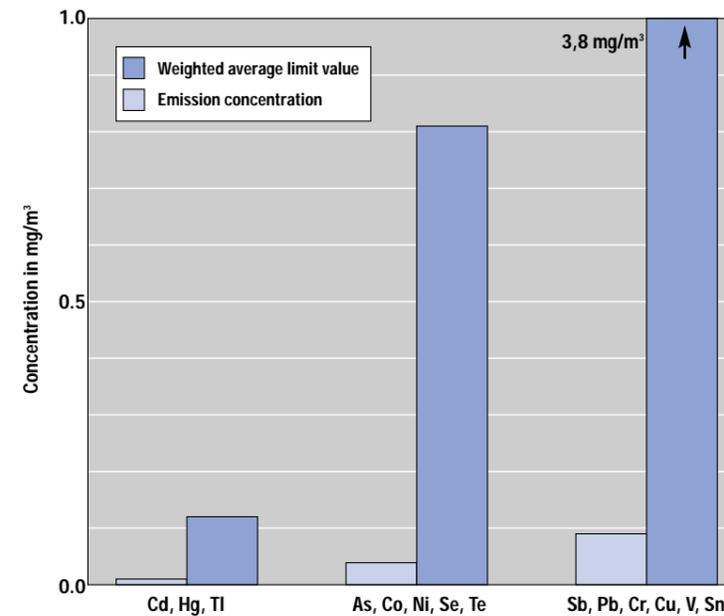
Fig. 10 Comparison between permissible emission concentrations of individual heavy metals and their average contents in the exhaust gas of a particular kiln plant taken as an example
