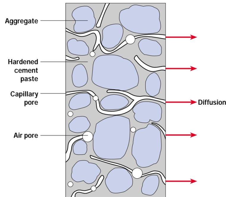
Fig. 7 Structure of concrete: hardened cement paste, aggregates, capillary pores
