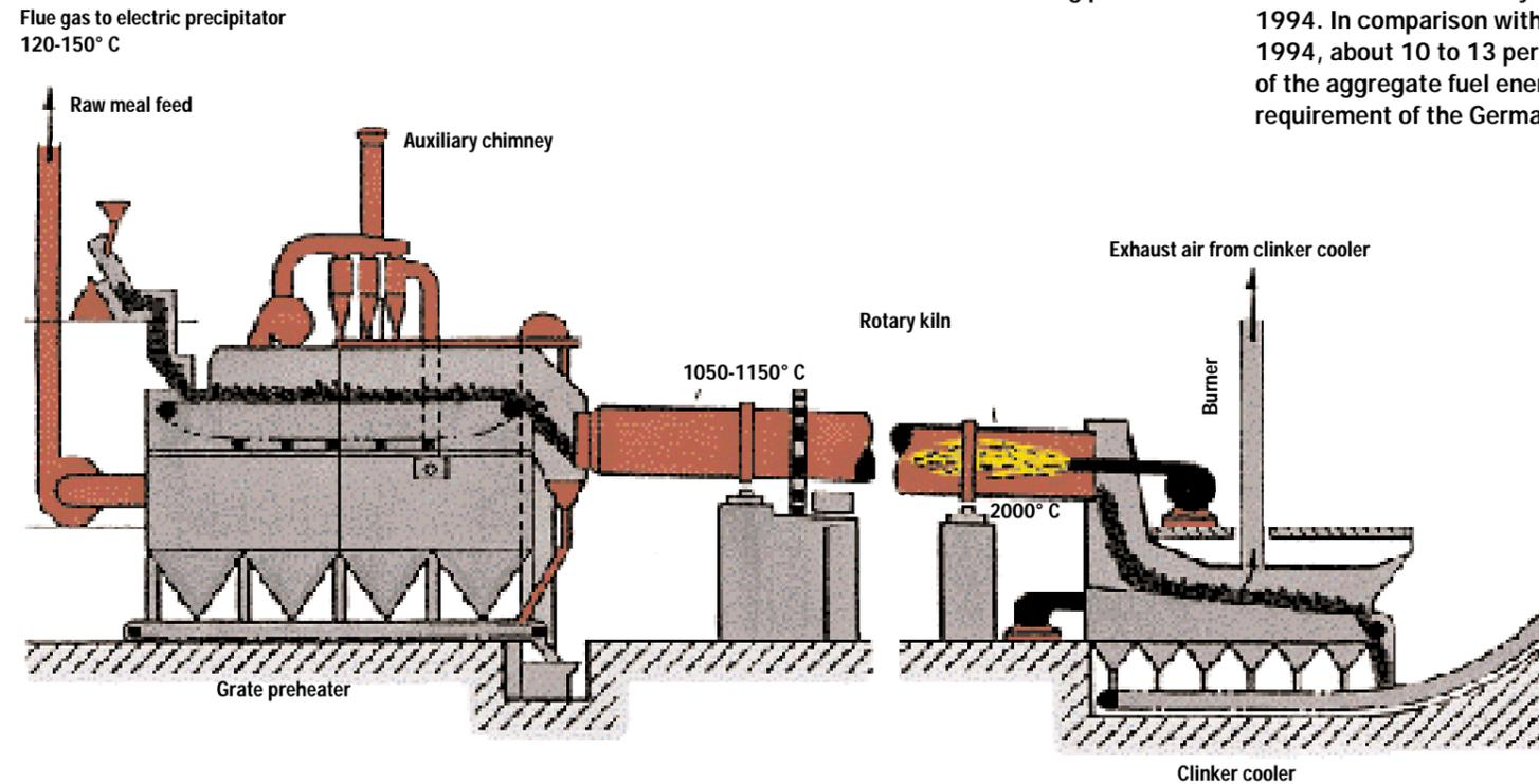
Fig. 4 Rotary kiln plant with grate preheater (Lepol kiln)
