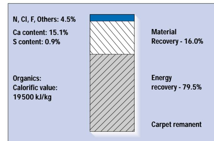
Fig. 12 Utilization of alternative materials in the clinker burning process based on the example of used tyres and carpet remanent
