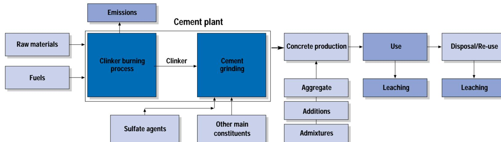
Fig. 6 Life cycle of cement and concrete
