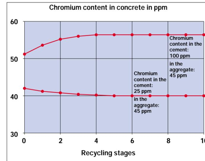
Fig. 14 uses the element chromium as an example to show the influence of repeated recycling on the overall content in concrete (proportion of recycled aggregate in this case: 50%). What is decisive is the contents in the cement and in the natural aggregate used. It becomes evident that the trace element content can both increase and decrease by re-use. In both cases the contents obtained range within the order of magnitude of concrete made using natural aggregate exclusively.
