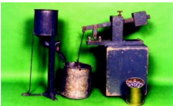
Fig. 1: Bending tensile test device of 1875
