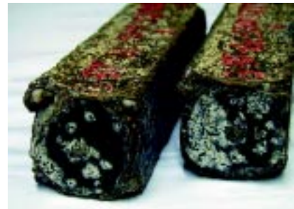
Fig. 2: Picture of a damaged concrete test specimen (standard prism) made of Portland cement with limestone chips as aggregate after 400 days' storage in sulphate-containing solution (29800 mg SO 4 /l) at 8 °C
