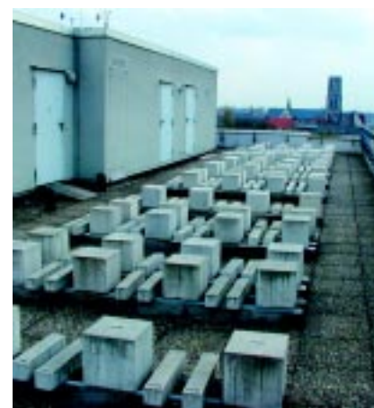
Fig. 1: Storage of concrete test specimens under practical conditions in the outside store
